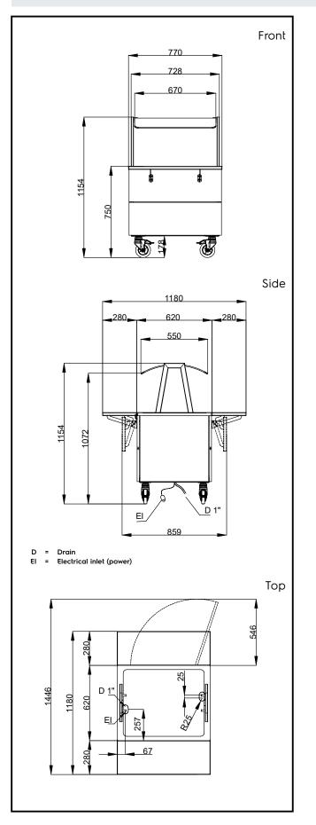
Flexy Compact Refrigerated well on cupboard, static with fan (2GN) with wheels, overshelf with LED lights, H=750mm The company reserves the right to make modifications to the products without prior notice. All information correct at time of printing.
